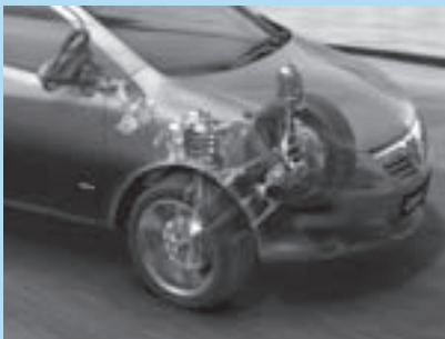
MacPherson strut front suspension.
