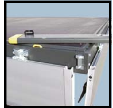
Removable rear corner post with tailboard restraint cords
