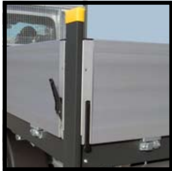
Flush fitting, discrete sideboard locks
