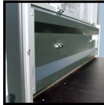
Four bulkhead load lashing points
